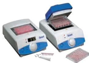
**Wide range of interchangeable blocks** – extraction tool supplied as standard for easy and safe removal of blocks
